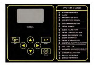
**Description** – Firetrol® combined automatic and manual Mark IIXG based diesel engine fire pump controllers are intended for starting and monitoring fire pump diesel engines. They are suitable for use with both mechanical and electronic type engines. The controller is available for 12 or 24 volt negative ground systems, using lead acid or Nickel-Cadmium batteries. The controller monitors. displays and records fire pump system information.
